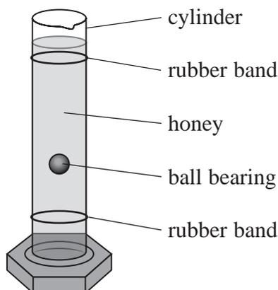
(a) The student placed rubber bands near the top and bottom of the cylinder. He started a stopwatch when the ball bearing passed the first band and stopped the stopwatch when the ball bearing passed the second band. He repeated this several times to determine a mean time.
