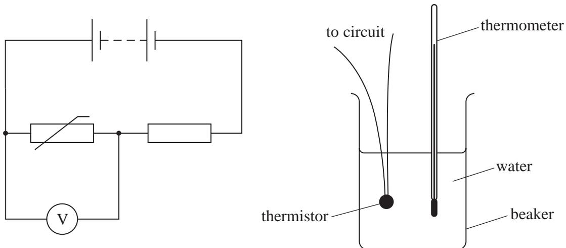
The student recorded  $\theta$  and corresponding values of the reading  $V$  on the voltmeter as the water cooled.
