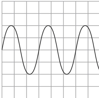
The time base of the oscilloscope was set to  $0.20 \text{ ms div}^{-1}$ .
