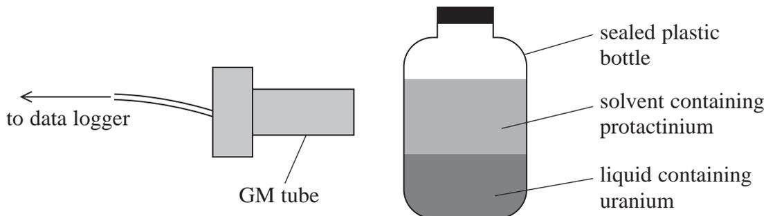
(a) Deduce whether alpha radiation or beta radiation from the inside of the bottle is detected by the GM tube.
