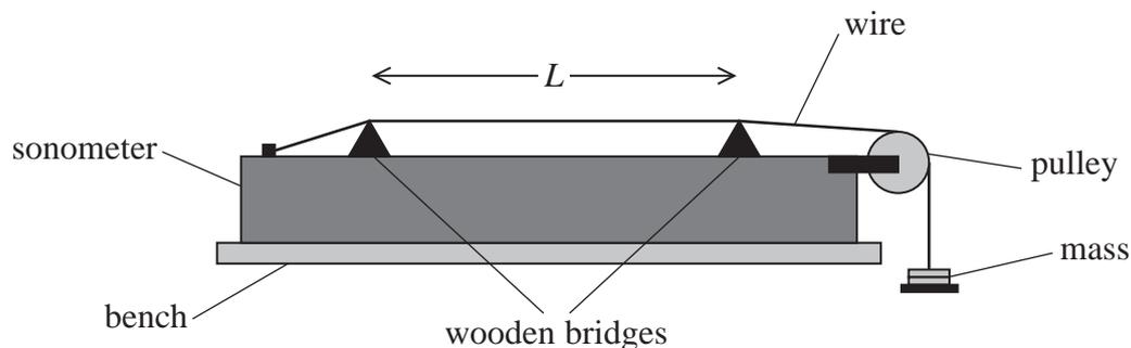
The student placed the base of a vibrating tuning fork in contact with the wire, at one of the bridges. This set the wire into oscillation. He adjusted the position of the other bridge until a single-loop standing wave was produced on the wire between the bridges.
